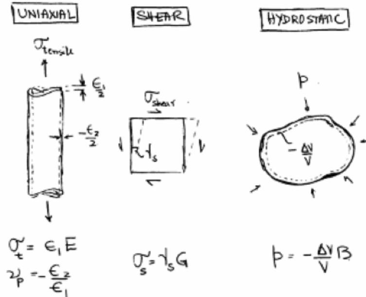
The Instron test is an example of uniaxial deformation.
