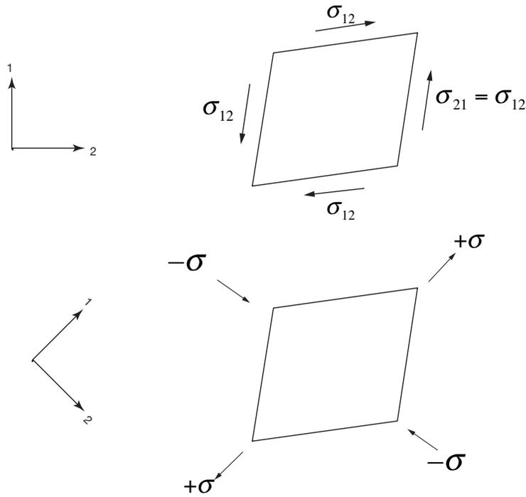
The principal stresses and strains for pure shear deformation are
