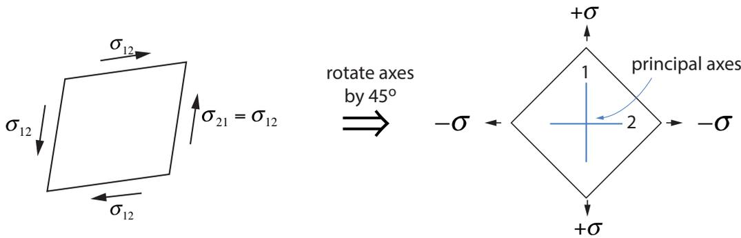
The stress and strain tensors using the principal axes are
