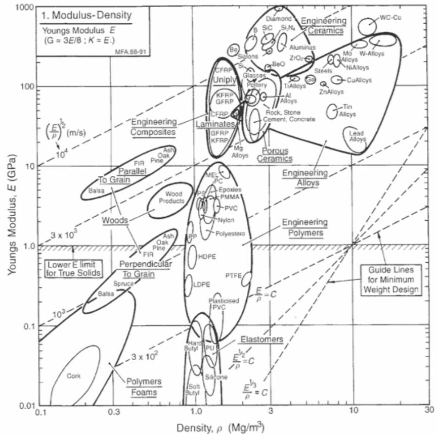
HW 01A.2: (i) Create a hierarchy of different materials classes in the order of increasing elastic modulus using the information given in the map on the right. (ii) Composites made from polymers and carbon fibers have their modulus closer to that of carbon. Can you model the modulus of the composite made with 70/30 carbon/polymer mixture (by vol). (iii) Which material would you use for making a diving board - explain why?
